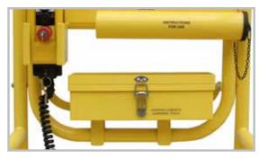
Width of gate reduced to prevent trapping of fingers as shown below.
