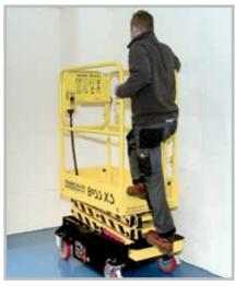
On entering the platform, ensure that the gate is closed behind you, as shown below.
