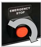
There is also an emergency stop button on the base unit. Push in to activate and twist clockwise to release
