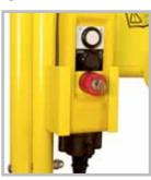
are adjacent to the machine. After a time delay and when the operator is sure it is safe to do so, the 'DOWN' button can be depressed a second time to continue the descent.
